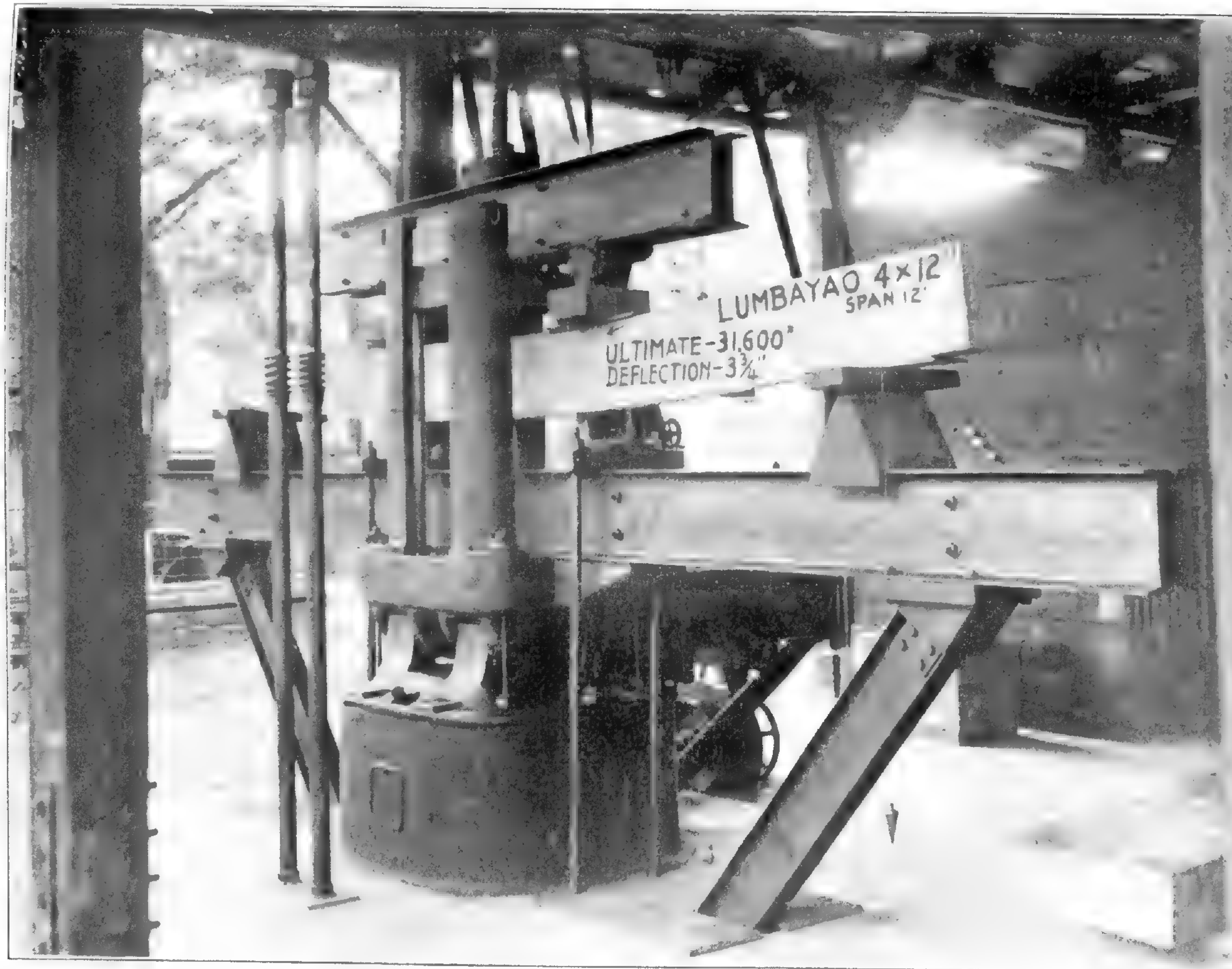
PLATE 1. TESTING MACHINE EQUIPPED FOR TIMBER TESTING.
